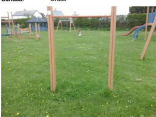
The item of equipment has a fall height exceeding 1.50 metres and grass has been provided as a safety surface Finding:
