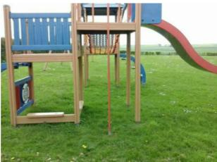
The item of equipment has a fall height exceeding 1.50 metres and grassmats are buried potentially affecting their impact attenuating properties. Finding:
