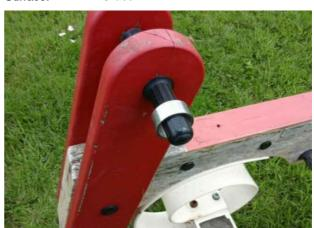
Finding: The end of handgrips and/or footrests have a cross section of less than 15cm2 and fail to meet the requirements of BS EN 1176:2008 Part 6
